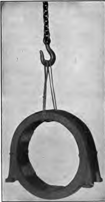
FIG. 30.—Hitch with one cable equalizing strain on four parts.
